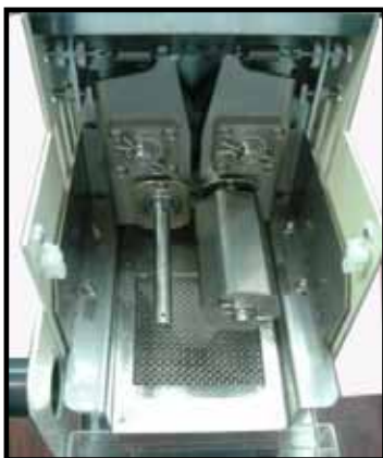
Hexagonal rollers can be easily detached for cleaning
