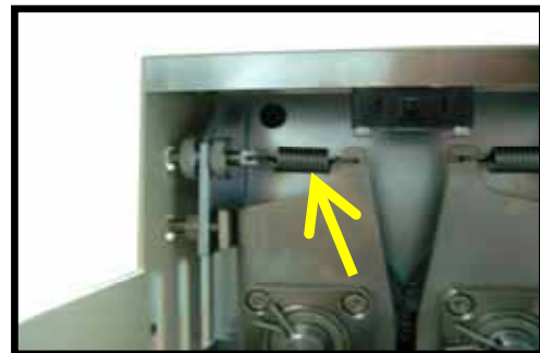
By adjusting the strength of spring or exchanging it, it will be easier to crush the soil, including the pebbles.
